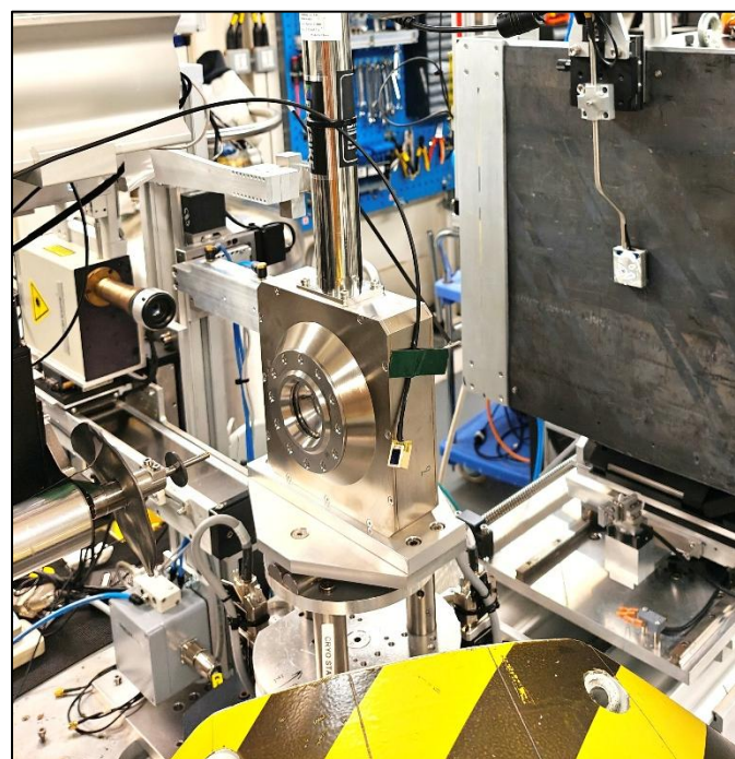
Figure 1: Cryostat on the diffractometer of I15 beamline
